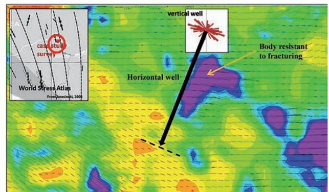
Figure 14 Seismic-derived anisotropy orientation compared to a rose diagram from well, and to information from microseismic monitoring of fracturing.
