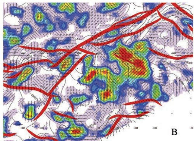
Figure 13 Panel A: results of simultaneous inversion. Sweet spots were estimated by comparing relationships estimated in Figure 12 with results of simultaneous inversion. Panel B: zoom on composite, azimuthal anisotropy map: colours indicate intensity, and arrows – orientation of anisotropy. Faults are in red.
