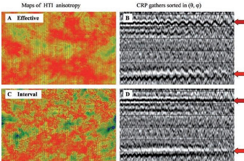
Figure 11 (A) – Map of effective HTI anisotropy for target (red arrow horizon). (B) – HTI anisotropy seen at the bottom of the overburden (brown arrow horizon) and at the target (red arrow horizon). (C) – Map of interval HTI anisotropy estimated for interval between horizons marked with two arrows. (D) Overburden azimuthal anisotropy compensated with full-azimuth PreSDM, and a clear decrease seen for the target horizon in this sample CRP gather.
