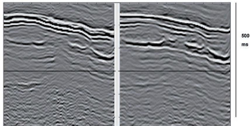
Figure 8 Sample sections of PreSTM (left) and full-azimuth PreSDM (right) images of the lower Permian model: section of the Zechstein. PreSDM image from depth was scaled to time for comparison.
