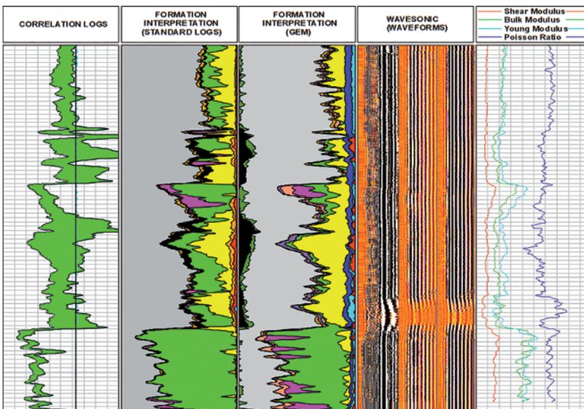
Figure 5 Sample of the final results of litho-facial analysis of the reservoir interval, based on standard measurements and GEM tool. Shale contents, porosity, hydrocarbon contents, and TOC (from the Passey method) were estimated. The two rightmost panels come from the cross-dipole sonic tool.
