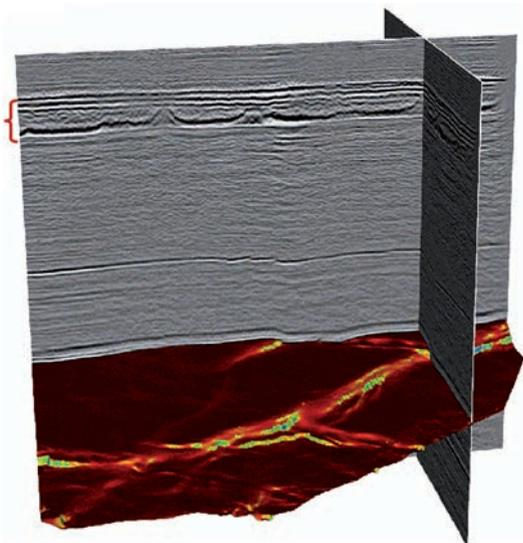
Figure 2 The complex Zechstein model causes deformations of the target Ordovician horizon. The brown brace points at the Zechstein interval with anhydrite barriers interlaced with salt structures.
