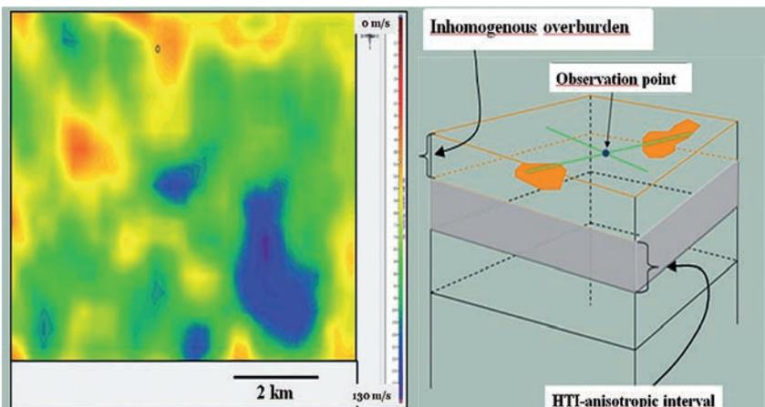
Figure 7 Full-azimuth tomography: model of overburden heterogeneities (horizontal slice seen on the left) was identified and separated from azimuthal anisotropy. The right side of the figure shows how velocity heterogeneities can be mistaken for velocity azimuthal anisotropy.
