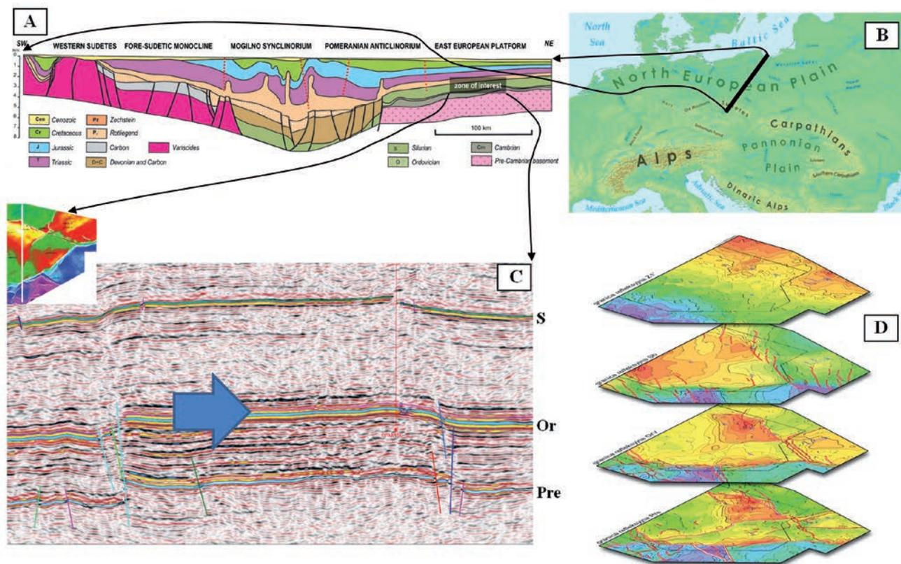
Figure 1 Survey area. Figure 1C shows a sample vertical section of the area; a depth map of the target horizon is in the top-left corner of Figure 1C. Regional cross-section in Figure 1A is after Karnkowski, 2008 and Zelazniewicz et al., 2011.
