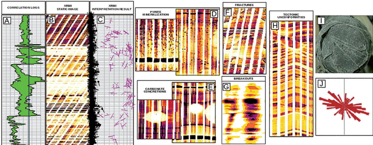
Figure 4 Sample of direct images of fractures recorded with XRFMI imager (panels B to H): D – pyrite, F, H – fractures, E – concretions, G – breakouts. In panel I - the core slice with natural fractures is displayed. Panel J shows a rose diagram of acoustic anisotropy in the target interval.
