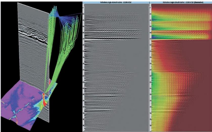
Figure 6 Compensation for irregular illumination. Detailed interactive analysis of rays and their attributes. Ray fan filtered with real acquisition geometry is investigated (A). Samples of seismic CRP gather (B) and CRP gather with illumination in colour (C).
