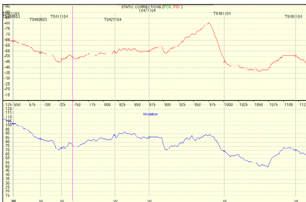
Fig.2. Display of receiver statics vs. elevation along with intersections marked
