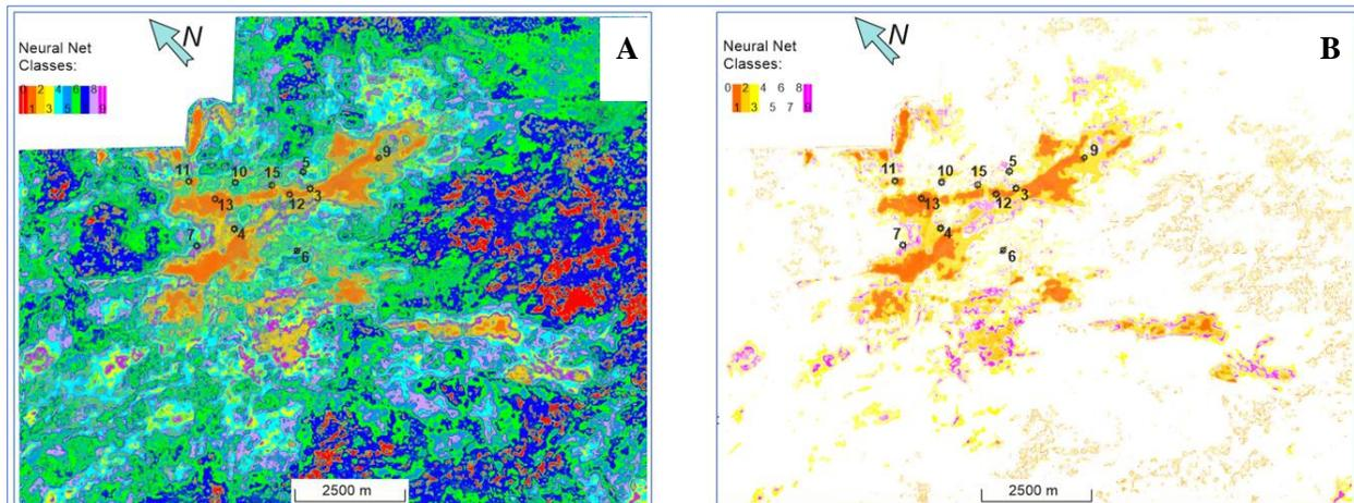
Figure 10. A box probe with manipulated transparency: resulting 10-class volume after applying Neural Net 3D algorithm (A), the selected classes well define the main channels of the studied complex (B).
