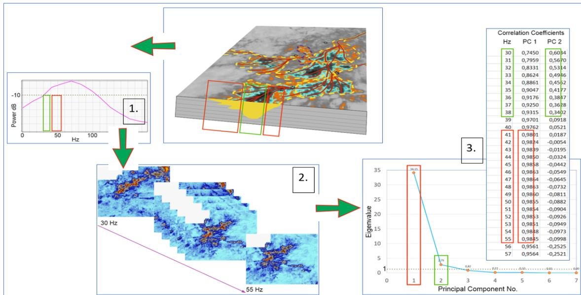
Figure 9. Generalized workflow for frequency data analysis.
