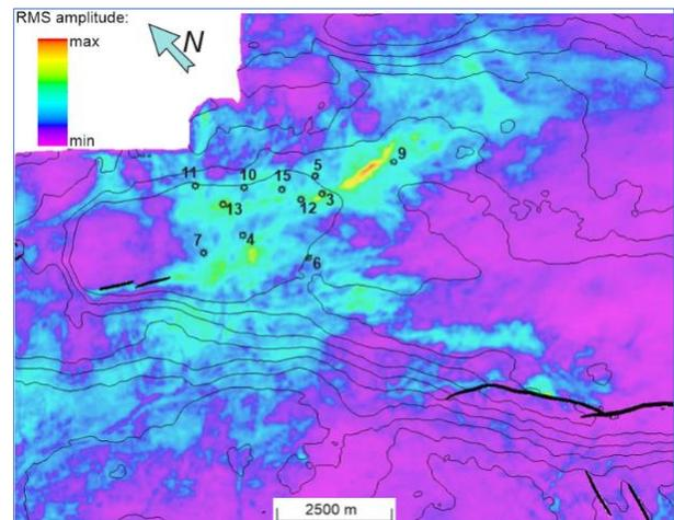
Figure 4. RMS seismic amplitude values distribution map.
