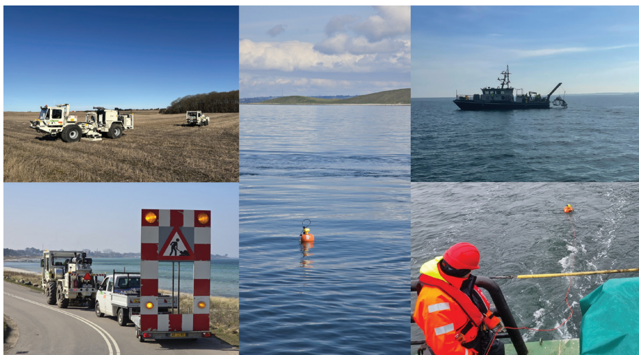
Figure 7 Overview of seismic survey operations. Left side – onshore operations: a heavy vibrator operating in a field and a mini vibrator working along a coastal road in Havnsø. Right side – offshore operations: one of the source vessels and node on the buoy deployment process. In the middle – a node mounted on a buoy. Photo credit: Karim Souissi, Ionut Popa, Mariusz Wisnowski, Branislav Berger.
