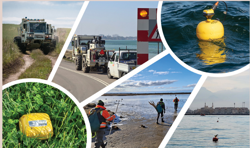
Figure 2: Seismic transition zone surveying includes vibrator operations, onshore data recording by nodes, and offshore data recording by nodes mounted on buoys and surveyors working along the beach.
